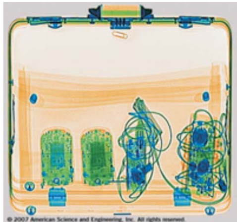
The dual-energy transmission image displays a laptop computer
